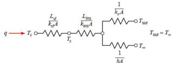
The total thermal resistance needed to achieve the desired heat loss rate is found from
