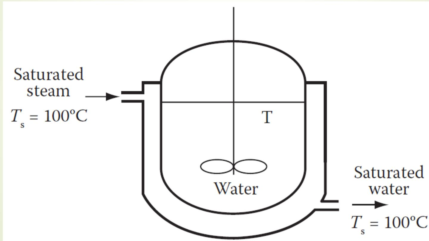
Heating of water in a jacketed, stirred vessel
