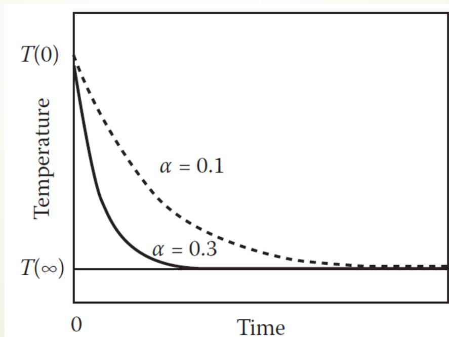
Graph of temperature vs time with two different values of  $\alpha$
