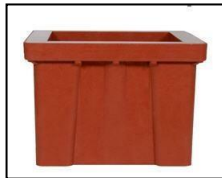
Figure 3. 2 Concrete mold with dimensions of 150×150×150 mm 3
